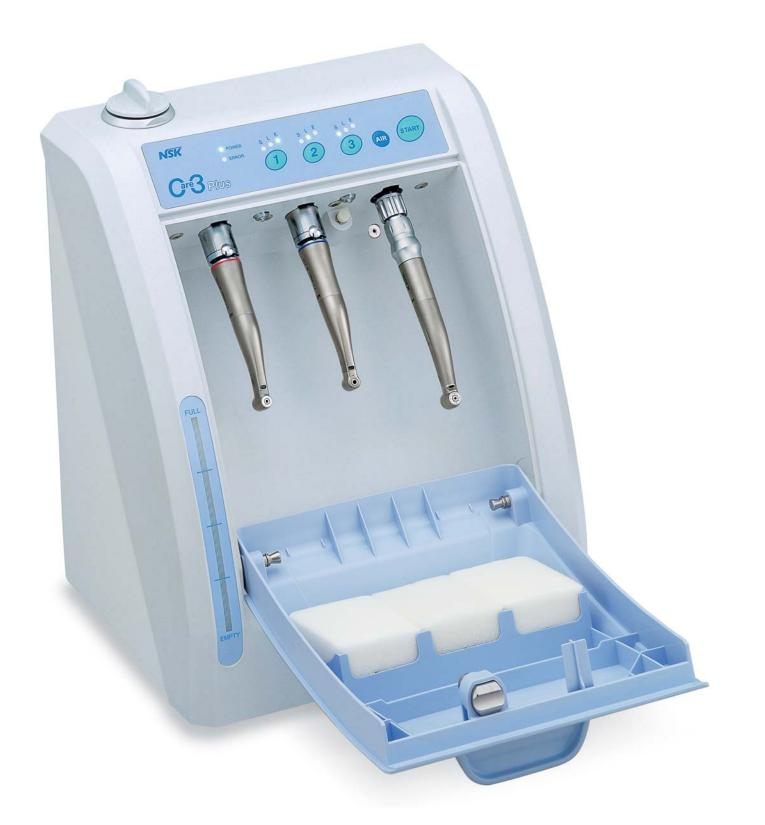
Correct maintenance performed at regular intervals is a key to high performance and longer life of your handpieces. NSK designed easy-to-use Care3 Plus to facilitate handpiece maintenance at your office. Care3 Plus automatically cleans and lubricates up to 3 handpieces at one time with a touch of button. Both high speed and low speed handpieces are processed thoroughly in a single 2-minute operation cycle.
